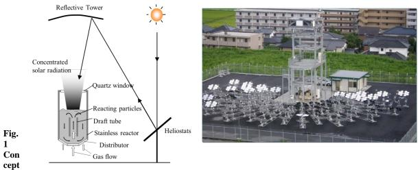
of solar thermochemical reactor with particles fluidized bed (left) and the novel beam down solar concentrating system for its demonstration (right).
